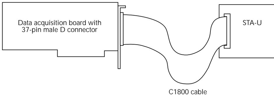
**WARNING** The maximum voltage allowed for a C1800 cable is 30V RMS, 42.4V peak, or 60VDC. Exceeding this limit could cause an insulation failure and shock hazard.
